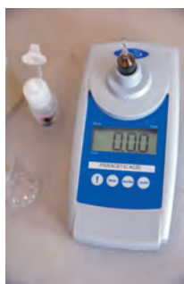
A peracetic acid (PAA) monitor is used to determine the amount of PAA needed for wastewater disinfection.
